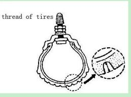
It is dangerous to use the wear tires; it will affect the traction, stability, steering and operating system. A new front tire should be replaced when the depth of thread is decreased below 1.6 mm. A new rear tire should be replaced when the depth of thread is decreased below 2 mm.
