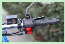
ENGINE STOP SWITCH (1) Press the " (1) "the electricity can be connected and the engine can work. It is of a emergency stop switch. If the button is on " (2) position, the engine can not work, the starting electricity is totally cut off
