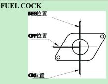
This type of motorcycle is equipped with manual acting fuel cock. There are three positions: "ON", "RES" and "OFF".
